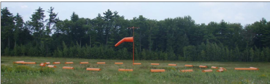
Figure 6-32. Segmented circle and wind cone
