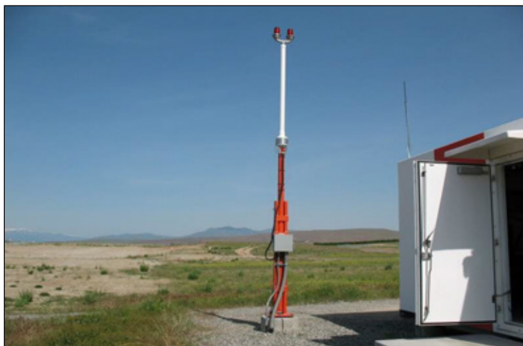
Figure 6-25. Distance Measuring Equipment (DME) antenna
