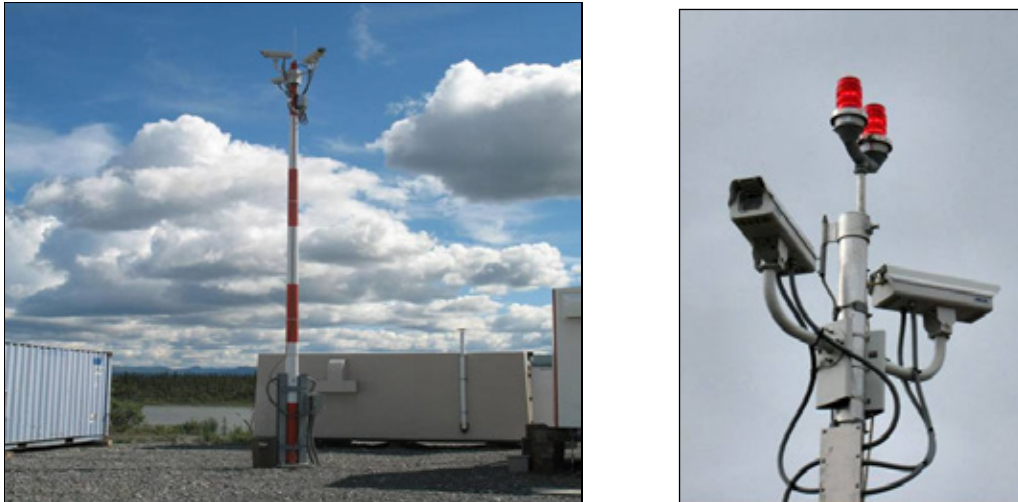
Figure 6-34. Weather Camera (WCAM) pole
